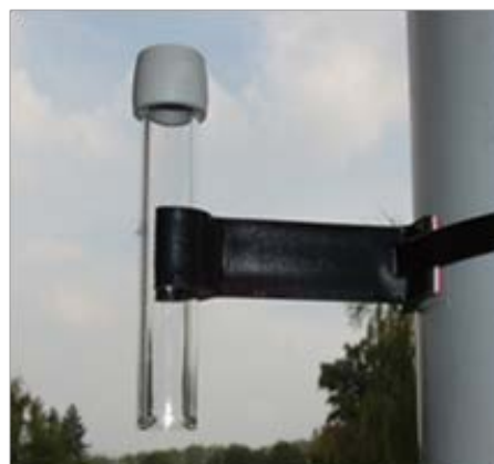
Figure 3: Diffusion tube to measure NO 2 in situ.
