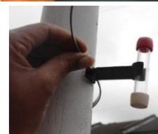
sample is placed at breathing height. In most public places this may not be feasible; to reduce loss or theft, it is recommended that tubes are placed at a height of 1.5-2m on public thoroughfares. **Remember**, the further away from the road, the less likely your readings will reflect the levels you are exposed to whilst walking around your community. Note, Defra guidance on height recommends 2-4m (this recommendation is based on standardizing for comparison across sites
