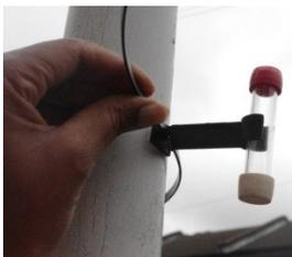
**LOCATE:** Select a suitable site to position the diffusion tube. If you are doing this as a community monitoring project then divide the area up into 200m grid squares and take a couple of samples in each of the grids to get a good coverage of the area
