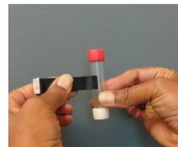
**FIX** sample in a secure position in the selected location. Make sure: there is free circulation of air around the tube and that they are positioned more than 10m away from air conditioning outlets, extractor vents or heater flues.
