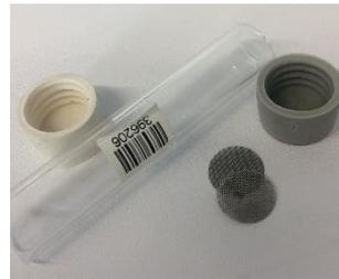
NO<sub>2</sub> using a steel mesh coated with a chemical called triethanolamine (TEA), which is located at the end of the tube with the grey stopper, see
