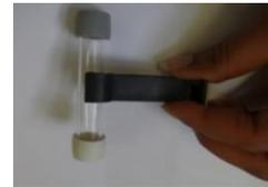
**SAMPLE:** On the coordinated start day, once in position, remove the **WHITE** cap which should be facing **downwards**. **DO NOT REMOVE THE GREY CAP** (you should see the absorber- small mesh inside the tube, beneath the grey cap). Leave tube in position for the 4-week exposure period, or until the specified changeover day. Remember to keep the white cap in a safe place as you will need to replace this to return the tube for analysis.
