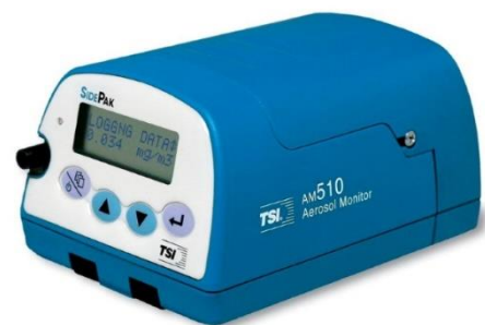
Figure 5: Sidepak Aerosol Monitor to measure personal exposure to particulates
