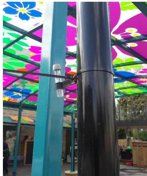
Figure 4. Monitoring sites hosting diffusion tubes to monitor nitrogen dioxide
