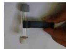
**SAMPLE:** On the coordinated start day, once in position, remove the **WHITE** cap which should be facing **downwards**. **DO NOT REMOVE THE GREY CAP** (you should see the absorber- small mesh inside the tube, beneath the grey cap). Leave tube in position for the 4-week exposure period, or until the specified changeover day. Remember to keep the white cap in a safe place as you will need to replace this to return the tube for analysis.
